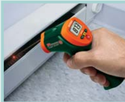
Test for temperature in heating systems
