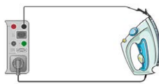
Earth bond test
