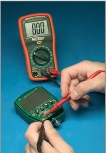
Integrated Non-Contact Voltage Detector for quickly checking the presence of live wires before testing.
